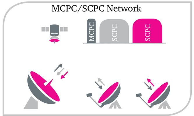
High-speed UHP SCPC modems allow creating dedicated channels of any purpose and throughput. It could be classic “point-to-point” SCPC channels of any asymmetry or “point-to-multipoint” MCPC broadcasting or even multi-site network based on combination of MCPC and SCPC channels.
